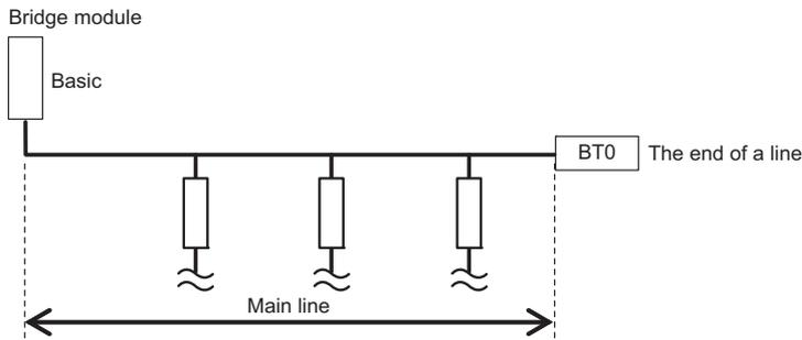
**Important** Connect a terminating resistor at the end of a line for one bridge module.
