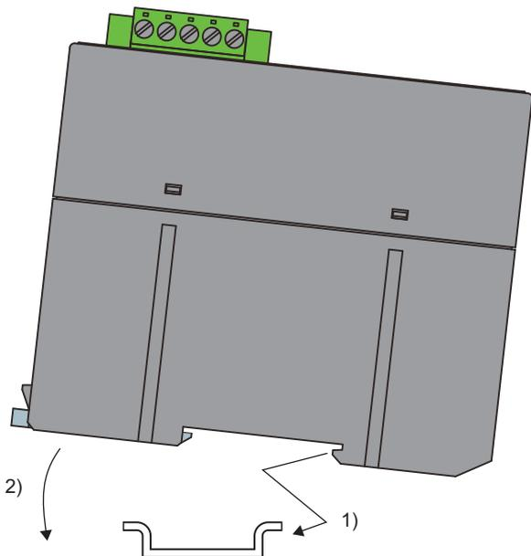
1. Hook the upper fixing tab on the bottom of the module to the DIN rail.
