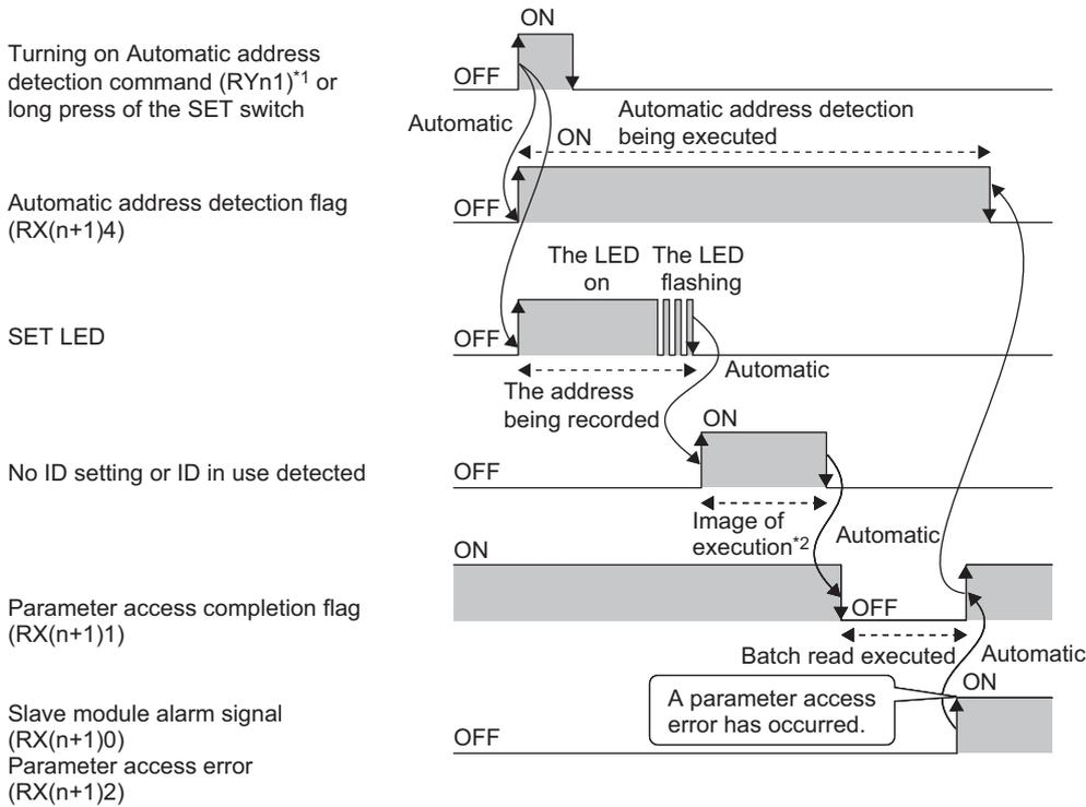
\*1 When turning on Automatic address detection command (RYn1), Automatic address detection command (RYn1) must be turned off after checking that Automatic address detection flag (RX(n+1)4) turns on and the SET LED is on.
