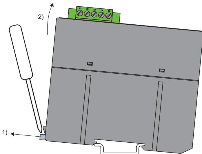
1. Insert a flathead screwdriver into the hook and pull the hook to remove from the DIN rail.
