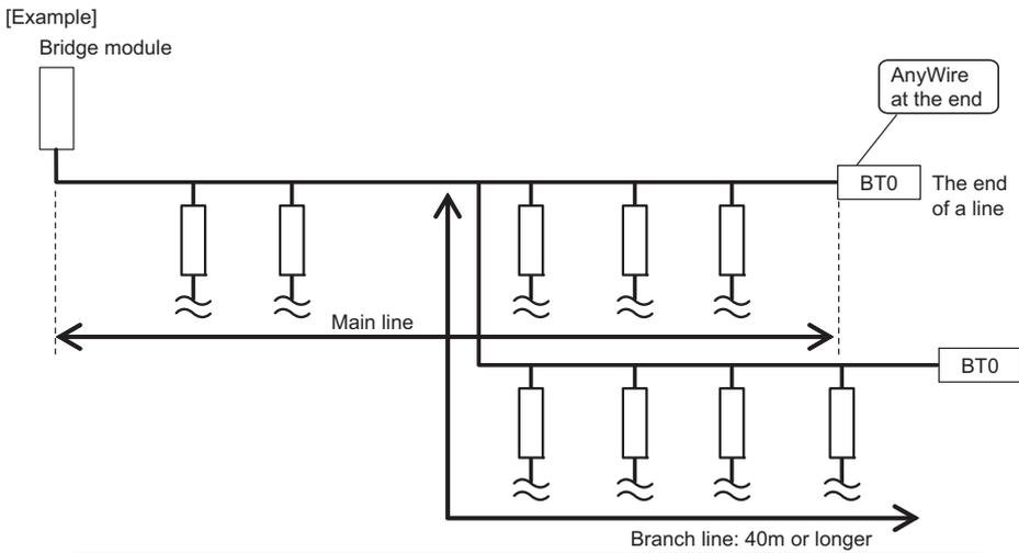
**Important** Connect one terminating resistor at the end of a branch line that exceeds 40m. Three terminating resistors can be connected in total in the AnyWireASLINK system.
