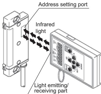
In the slave module, an address between 0 and 254 can be written. (This number is not an ID value.) Do not set 255 to the address. Doing so will cause a No ID setting error.
