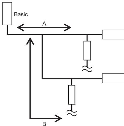
The total length of the transmission distance for the AnyWireASLINK system can be calculated from  $A + B$ . Note that the total length should not exceed the maximum transmission distance set for the system to branch lines.
