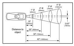
sured, excluding the surroundings. Remember that the measurement size is one-tenth the distance to the target. For example, if the thermometer is at 10", then the size measured is 1".
