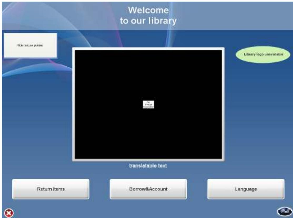
To display the self-service screens in admin mode click on logout from the remote admin screen. You will then notice the “hide mouse button” on the top right hand corner. This allows the mouse cursor to be visible. If you click or press this button the system will remove the mouse cursor and exit admin mode. You will need to rescan the admin card and then confirm and logout again. Once in this mode all GUI settings can be changed.
