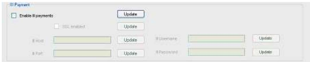
This section is only used for Triple III web based payment systems. Tick enable III payments and fill in the correct details, these will be given by the LMS supplier (Triple III)
