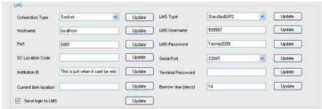
The above configuration is for the LMS connection via SIP2. The details of the connection should be given to you by the LMS. If you are unsure what settings should be added to this section, please call the D-Tech helpdesk for advice.
