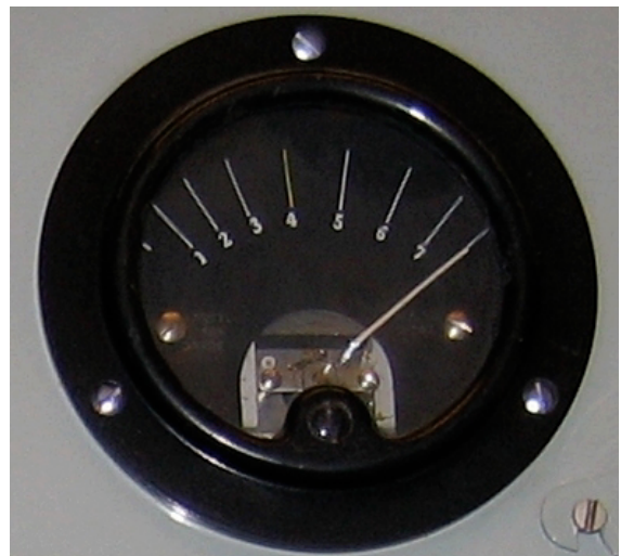
"Nation Shall Peak Six Unto Nation" An old style PPM with right-hand mechanical zero, as used with valve equipment (switched off when photographed) source: Wikipedia.
