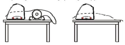
6.2.2.3 Adjust horizontal position of paperweight wheel according to width of paper. A distance of mini mum 1-10CM is set between paper-weight wheel and paper edge to ensure good running of paper.(note: the paper-weight wheel can not press on bearing).
