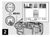
→ Press MENU and select [DELETE] with A/▼ on the control button, then press ●.
