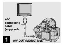
Connect the A/V connecting cable to the A/V OUT (MONO) jack of the camera and the audio/video input jacks of the TV.
