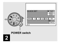
→ Slide the POWER switch in the direction of the arrow to turn on the power.
