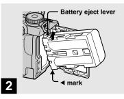
→ Install the battery pack, then close the battery/"Memory Stick" cover.
