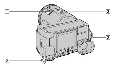
Attaching the lens cap and the shoulder strap.
