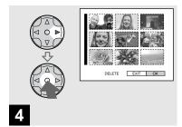
→ Press MENU and select [OK] with ▶ on the control button, then press ●.
