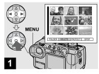
While an index (nine-image) screen (page 34) is displayed, press MENU and select [DELETE] with ◄/▶ on the control button, then press ●.
