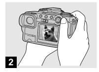
→ Hold the camera steadily with both hands and position the subject in the center of the focus frame.
