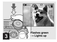
Press and hold the shutter button halfway down.
