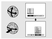
To change the current settings of the camera, bring up the menu or the SET UP screen (page 42), and use the control button to make the changes.
