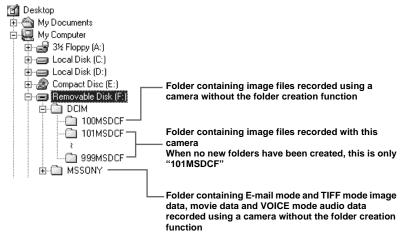
Data in the "100MSDCF" or "MSSONY" folders is data recorded using a camera without the folder creation function. These folders are for playback only, and your camera cannot record images in these folders.
