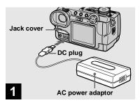
Open the jack cover and connect the AC-L10A/L10B AC power adaptor (supplied) to the DC IN jack of your camera.
