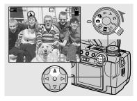
→ Set the mode dial to □, and press ▲ (‡) on the control button repeatedly to select a flash mode.
