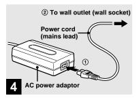
Connect the power cord (mains lead) to the AC power adaptor and then to a wall outlet (wall socket).
