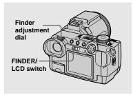
With the FINDER/LCD switch, you can choose to shoot either using the finder or the LCD screen. When you use the finder, the image does not appear on the LCD screen. Turn the finder adjustment dial until the image appears clearly within the finder, then shoot the image.
