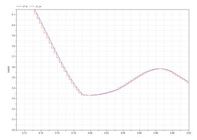
The blue trajectory is from the reference simulation and the red is from the co-simulation. Note that the latter is rendered as constant between the sample points.
