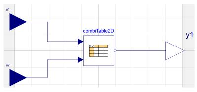
In the parameter dialog of combiTable2D, select **tableOnFile** to true, and propagate **tableName** and **fileName**. Give relevant default values for them. As an example, looking at the resulting Modelica code when having specified a table name and file name as default value, we find:
