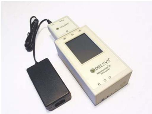
*Figure 8. The Main Unit connected to the Docking Module and the Power supply for charging purposes.*
