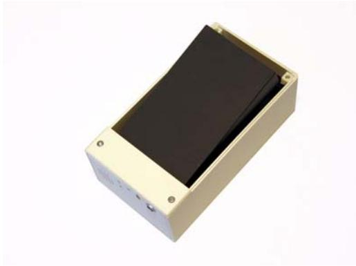
*Figure 13. Open the battery compartment at the back of the Myomonitor to replace the battery.*
