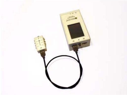
*Figure 9. Connecting the Main Unit and Input Modules via the Input Cable.*
