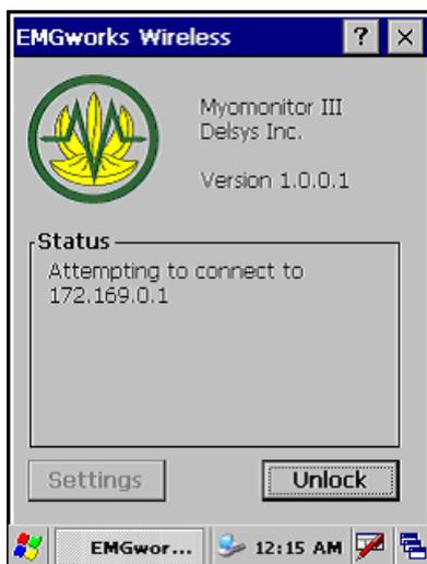
EMGworks Wireless will instantly attempt to connect to the default host computer on the Myomonitor network. If EMGworks Acquisition is running on the host computer and the network has been setup using the default parameters, the Myomonitor III should instantly connect.
