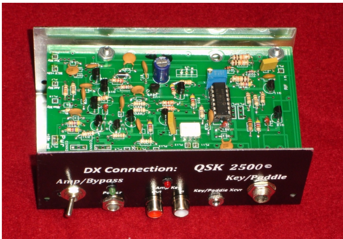
Figure 1a Delay potentiometer & jumper holes adjacent to PIC processor
