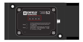
The S2 has 4 potentiometers (Responsiveness, Speed Damping, Force Damping, and Offset) which allow for maximum flexibility. A polymer non-conductive screwdriver is the preferred method for adjusting the potentiometers. Care should be taken not to allow metal screwdrivers to touch other components on the board.
