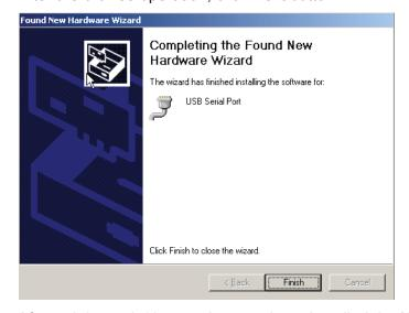
After 4.2.8 to 4.2.11 operation, you have installed the **USB Serial Port**.
