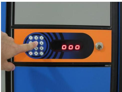
**STEP 2:** Control Unit enters the PIN-entry mode. Sign “Pin” is flashing on the Display Unit and beep acoustic signal is heard.
