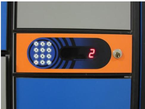
**STEP 3:** Indication of successful locking is the number of closed locker shown on Display Unit.
