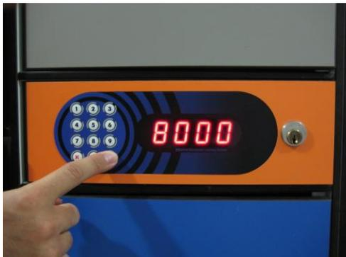
**STEP 1:** Enter group PIN code (number defined by “GrUP” parameter – from 8000 to 9999) to start multiple locking procedure and press the ✓ key.
