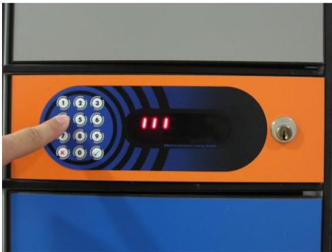
**STEP 3:** Type in a Master code (up to 16 digits). Signs “1” are displayed each time you press the key. Confirm the Master code with the ✓ key.
