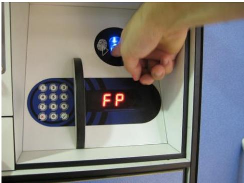
**STEP 2:** Sign “FP” is flashing on the Display Unit and beep acoustic signal is heard. Insert your finger in the Fingerprint module.
