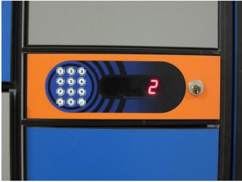
**STEP 3:** If correct PIN code is entered, locker number is displayed on Display Unit and corresponding locker is unlocked and opened.
