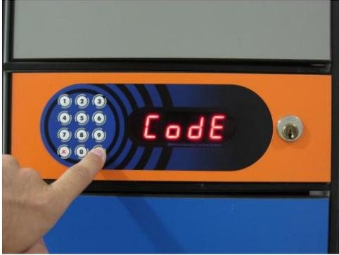
**STEP 2:** Sign “CodE” starts flashing on the Display Unit and beep acoustic signal is heard.
