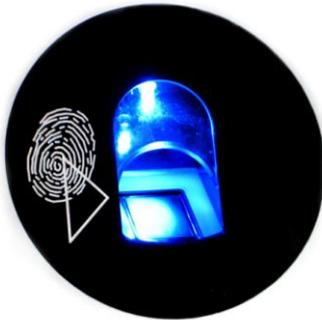
Fingerprint module allows users to lock/unlock the locker instead with PIN number simply by presenting the finger to sensor. It offers higher comfort for users as they don't need to remember PIN code. When fingerprint module is connected to ELS keypad control unit each user can freely choose whether he/she will lock the locker using fingerprint or PIN code.
