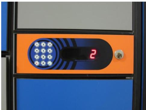
**STEP 6:** Locker number is displayed on Display Unit and corresponding locker is locked.
