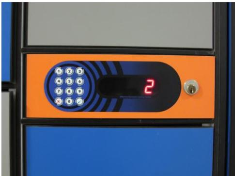
**STEP 3:** If correct PIN code is entered / fingerprint recognized, corresponding lockers start to unlock and open one after another and corresponding locker number is displayed on Display Unit.
