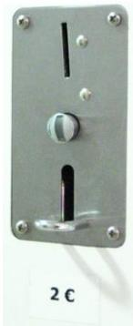
Control Unit ELS can be configured to ask for payment when locking the locker door. In that case Coin Acceptor is mounted near the Display Unit.
