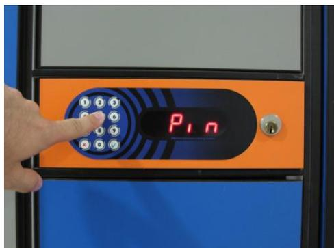
**STEP 2:** Sign "Pin" is flashing on the Display Unit and beep acoustic signal is heard. Enter the PIN code that was used to lock corresponding locker and confirm it with ✓ key.
