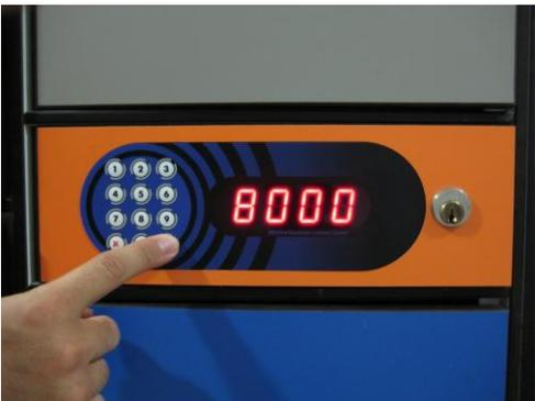
**STEP 1:** Enter group PIN code to start multiple unlocking procedure and press the ✓ key.
