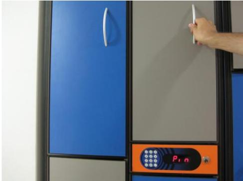
**STEP 1:** Close the locker door. Sign “Pin” is flashing on the Display Unit and beep acoustic signal is heard.
