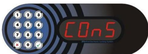
"ConS" message on Display Unit means that the Control Unit is in "construction mode" of operation. It is initialized with default parameter settings as it comes out of production.
