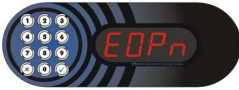
If emergency opening of all Lockers is initiated remotely by the network the system signals this by acoustic signal and displaying “EOPn” message for few seconds!
