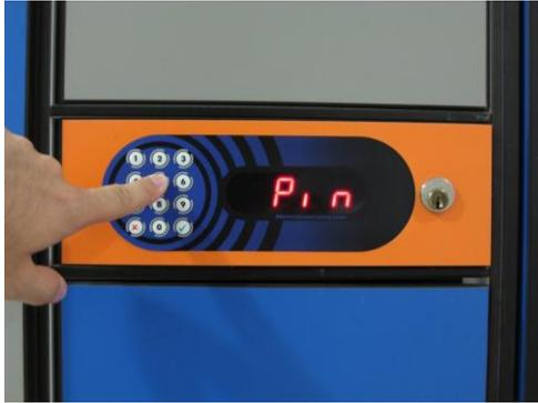
**STEP 2:** If PIN code was chosen sign “Pin” is flashing on the Display Unit and beep acoustic signal is heard. Enter the PIN code that was used to lock multiple lockers and confirm it with ✓ key.
