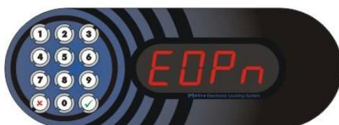
If remote opening of single Lockers is initiated over the network the system signals this by acoustic signal and displaying "EOPn" message followed by locker number.
