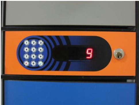
**STEP 2:** All the lockers connected to that Control Unit start to open one after another and corresponding locker number is displayed.
