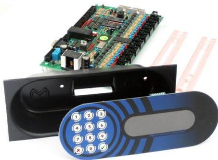
Control unit ELS Keypad is used in Metra Electronic Locking System (ELS) which is primarily designed and used for locking lockers.
