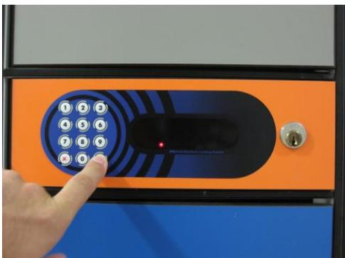
**STEP 1:** To enter Master mode press and hold the ✓ key for more than 2 seconds.
