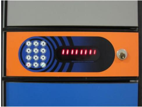
**STEP 3:** Control Unit enters MULTIPLE locking mode of operation indicated by time countdown on the display.
