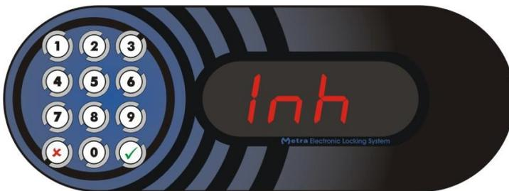
After 3 consecutive incorrect entering of PIN code / Master code, further attempts are blocked for 15 seconds. “Inh” (Inhibit) is displayed instead of flashing “Pin” / “CodE”.
