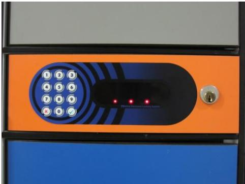
**STEP 4:** If correct Master code was entered the Control Unit turns to Master mode of operation. It is indicated by flashing 3 dots on the display.
