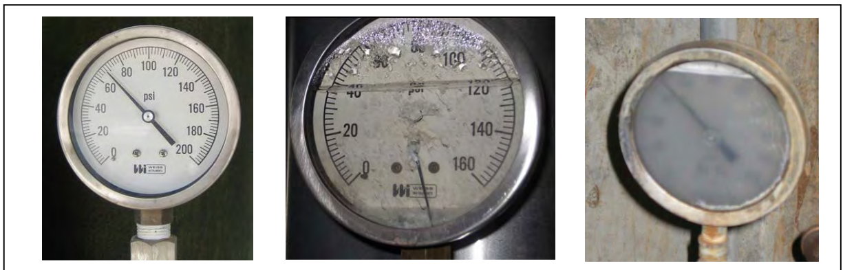
Figure 9 : Examples of a Clean Gauge and Two Visually Impaired Gauges
