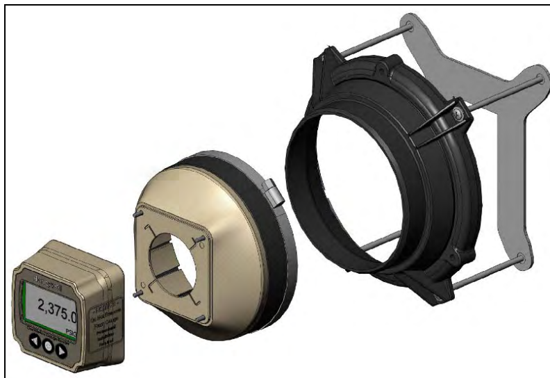
Figure 7 : Exploded View of a Process Gauge Mounting Adapter
