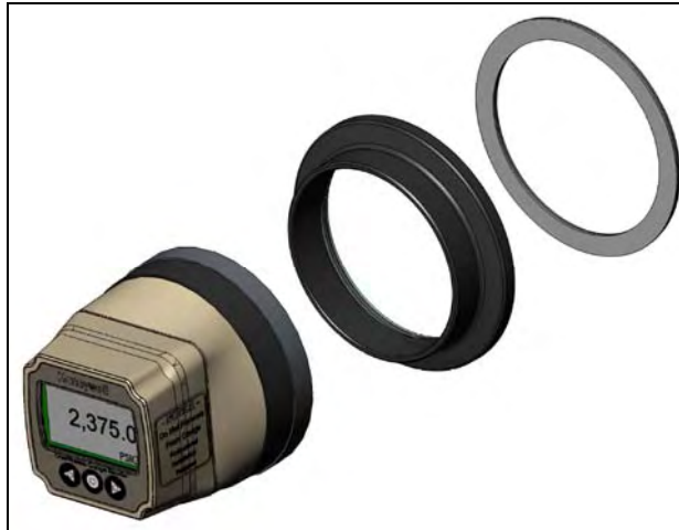
Figure 8 : Exploded View of Panel Mount Adapter
