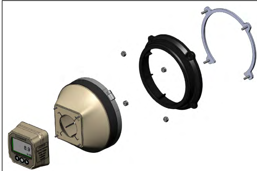
Figure 6 : Exploded View of Magnehelic/Photohelic Mounting Adapter
