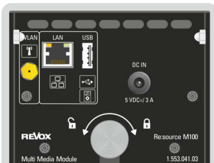
Rear view: Multimedia module with locking screw
