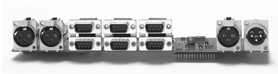
Figure 1.2 KP-32 connector option board.
