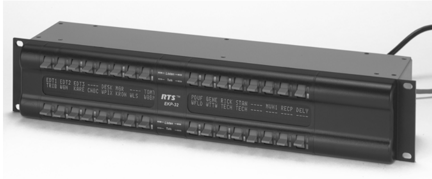
Figure 1.4 EKP-32 expansion keypanel front view.
