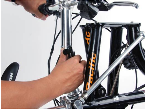
9. Fold the handle bar to the side by opening the stem locking lever. Rotate the lever rearward to release.
