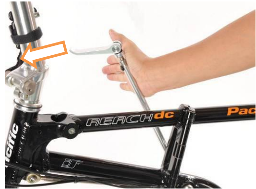
7. Secure the frame together by rotating the frame locking lever forward and down into the front connector.
