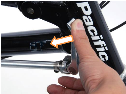
8. Securely lock the locking lever in place by securing the quick release clamp into the closed position.
