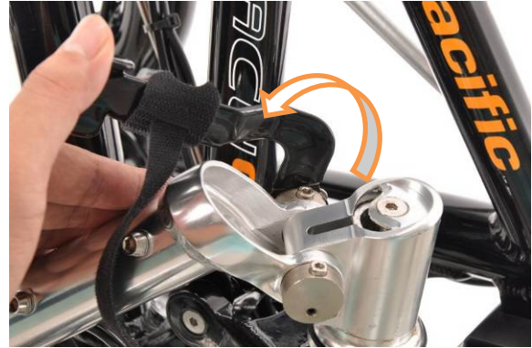
10. Return the stem locking lever back forward against the stem when the handle bars are folded.
