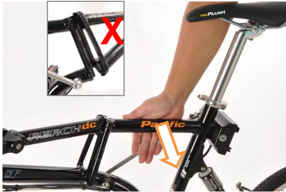
6. Use your right palm to push the top tube by the seat tube to put the frame into position. WARNING: Never place your hands and fingers inside the folding part / mechanism.
