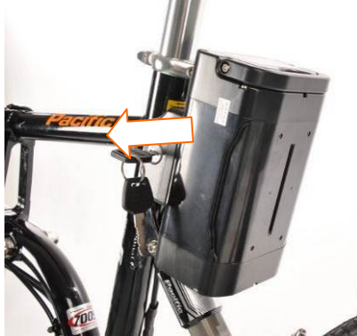
Turn key to 'lock-off' position. Hold battery pack case and pull left directly.
