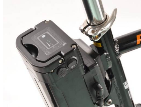
Electricity level display button. Recharge immediately when one red light is blinking.
