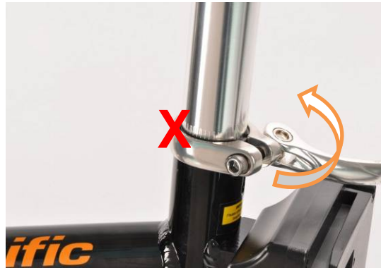
9. Adjust seat tube and clamp. Note: Do not raise the seat post higher than the minimum insertion mark.
