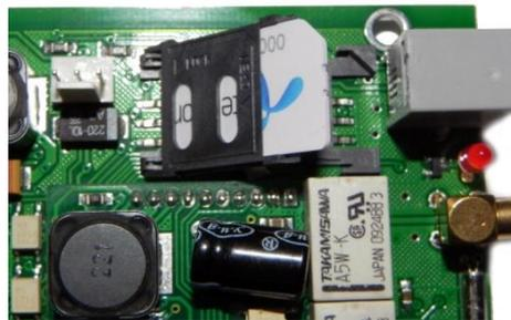
3. Put the given SIM-card into the SIM-holder bay (which is also activated with GSM/GPRS network data package option by the cellular network provider). You must be ensure the right SIM-card insertion direction with taking care about, the chip-side must be at underside.
