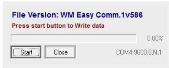
3. The download from the device started which can be checked with the progress indicators percentage status. When the configuration download was successfully finished the '**Communication Successful!**' message appears with a 100 percent status.
