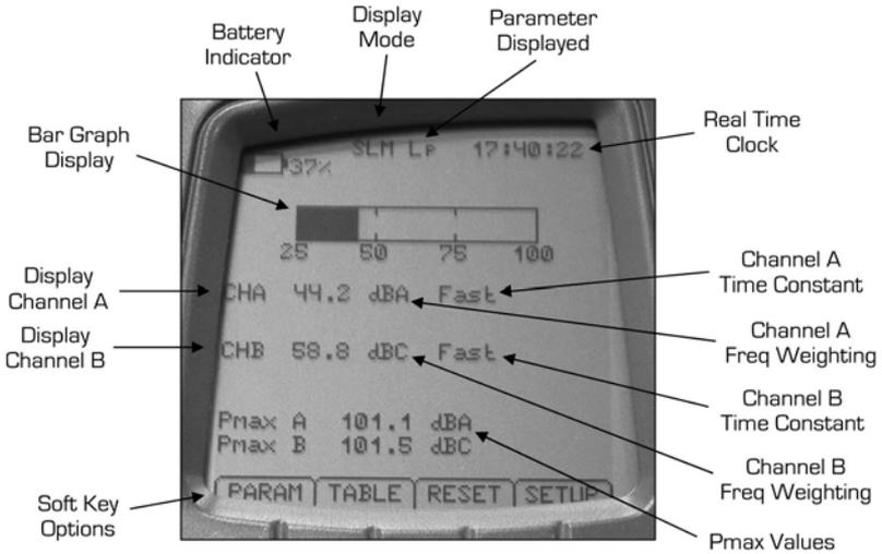
Figure 10 - SLM Mode Screen Layout
