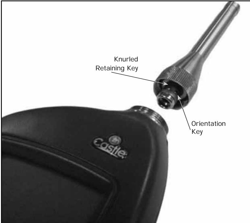
Figure 1 – Attaching the Pre-Amplifier with a Class 1 Instrument
