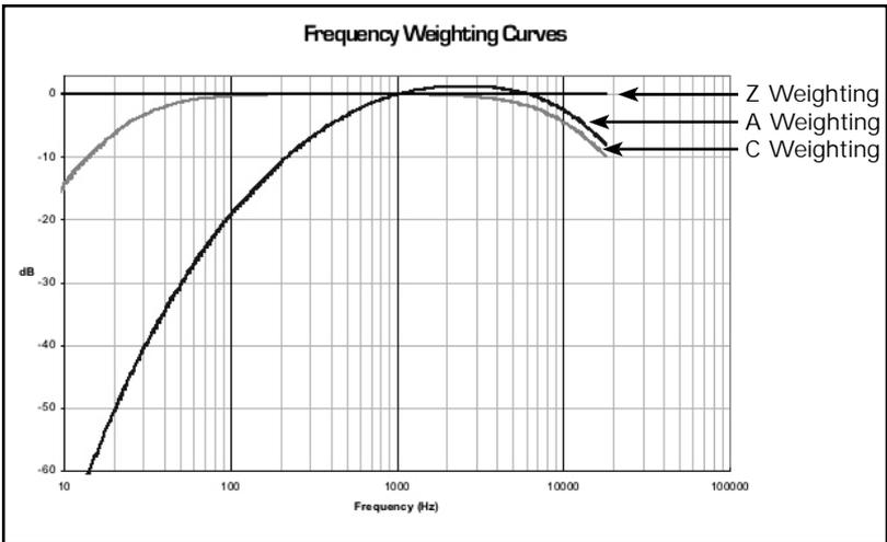
Figure 3 – Frequency Weighting Curves
