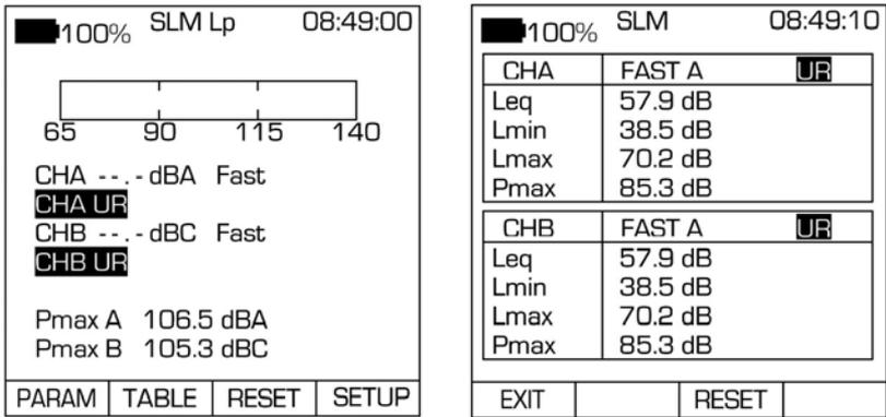
Figure 6 - SLM Mode Under Range Indicators
