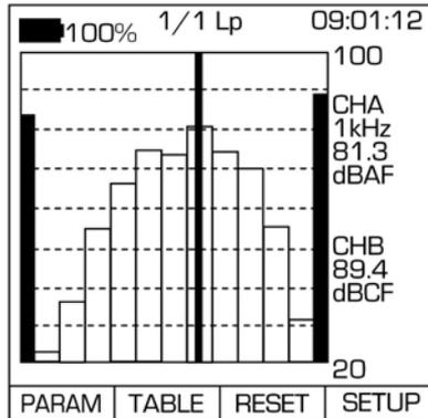
Figure 46 – Graphical Full Octave Mode Display Screen
