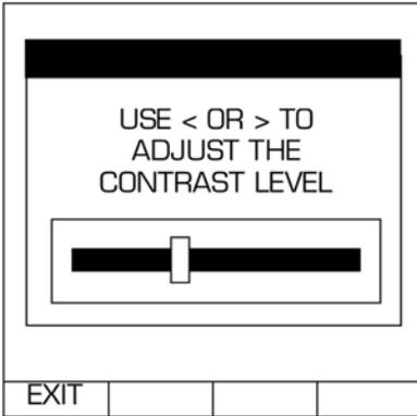
Figure 40 - Contrast Adjustment Screen
