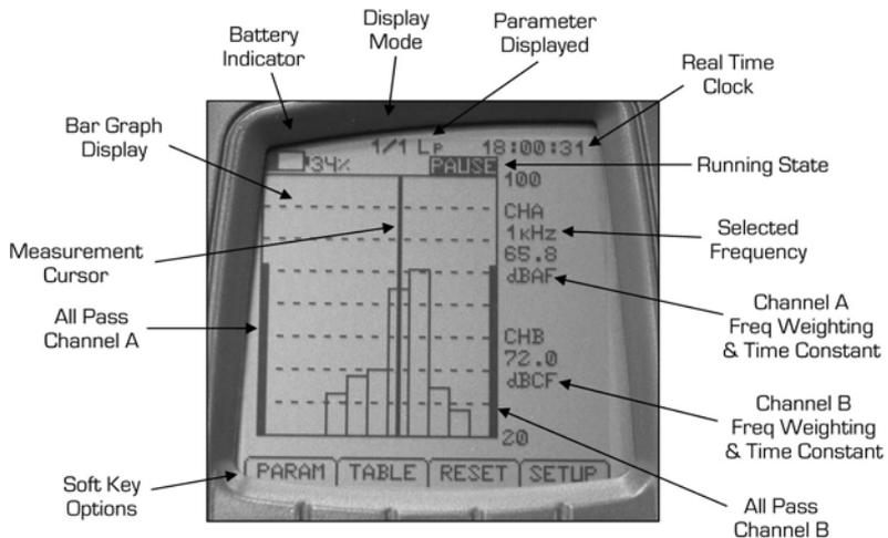
Figure 11 - Full Octave Mode Screen Layout
