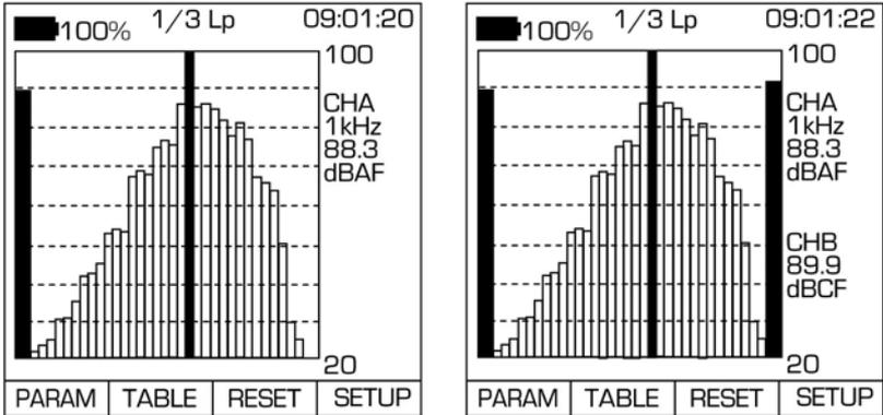
Figure 47 – Graphical Third Octave Mode Display Screen
