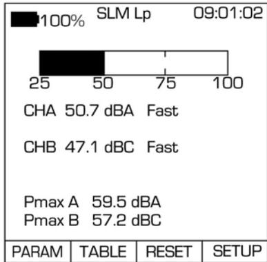
Figure 45 – Graphical SLM Mode Display Mode Screen
