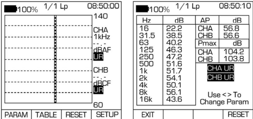
Figure 7 - Full Octave Mode Under Range Indicators
