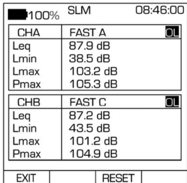
Figure 4 - SLM Mode Overload Indicators
