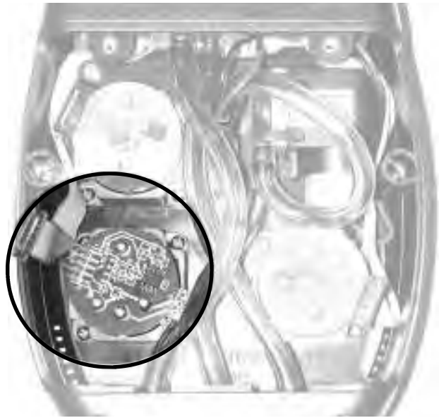
Fig. 4: Example of sensor with electrical connection removed.
