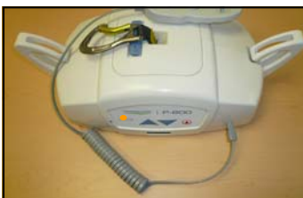
Figure 12E - Charger is connected to the lift. The indicator light on the charger will be ORANGE indicating that the lift is charging.
