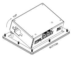
Remove the old battery\* from the holder and replace with the new battery. Replace the rear cover, cables, and re-apply power. Using DSI8000 or the unit's keypad, enter the correct time and date.
