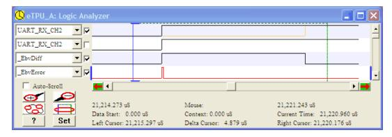
The check box to the left of each waveform is used to enable and disable display of the underlayed behavior verification data. The check box in the second waveform is unselected which is why the behavior verification waveform does not appear. Note that if no behavior verification data is loaded then no yellow waveform will appear, even if the behavior verification checkbox is enabled.
