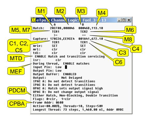
M1 and M3 are the Match register values for action unit A and B, respectively.
