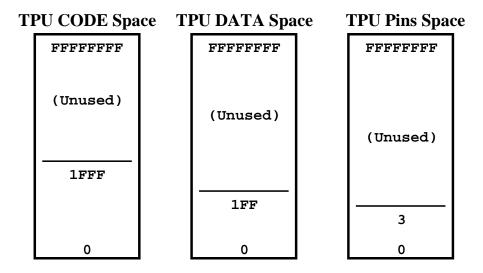
The TPU simulation model fetches code between 0 and 1FFF hexadecimal from its CODE space. It accesses its parameter RAM and host interface registers between 0 and 1FF hexadecimal of its DATA space. And it accesses its channel pins in the first four bytes of a simulated PINS space. Note that its code banks are "unrolled" and placed linearly in memory.
