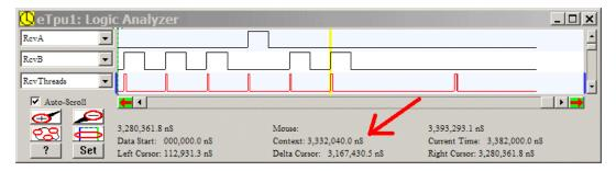
The window shown below is similar to the window set to the ARINC\_FX function, except that it is configured to show only the information from the channel named, "RcvA." Note that this name has been assigned to this channel in the test vector file using the NODE command, as defined in the test vector file section. Because it displays only the information from a single channel, it may not reflect the true worst case.
