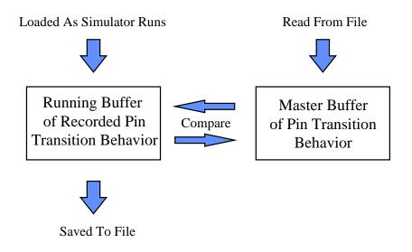
The running buffer is filled as the eTPU Simulator runs. Whenever a pin transition occurs, information regarding this transition is stored in this buffer, which is also used to draw the signals in the logic analyzer window. This pin transition information can be selectively recorded to file using the create\_ebehavior\_file("filename.ebv"), add\_ebehavior\_pin("<pin name>") and close\_ebehavior\_file() script commands; also see Enhanced Pin Transition Behavior Verification below.
