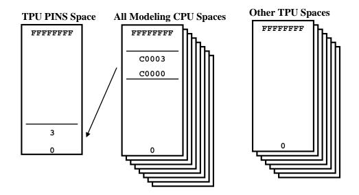
The following build script commands generate the address space transformations shown in the above figure. If the modeling CPU does a read from its address C0000 hexadecimal, the read will actually access the shared memory with the TPU in its PINS space.
