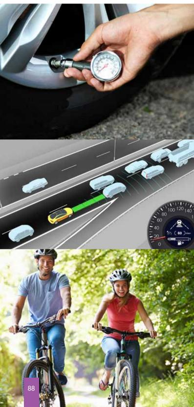
• The tire air pressure affects 5-10% of fuel consumption. 0.5 bar diminished increases fuel consumption by 5%. Pay attention to the air pressure value in tires are in recommended value. Let's prefer to use radial tires recommended for highways and urban.
