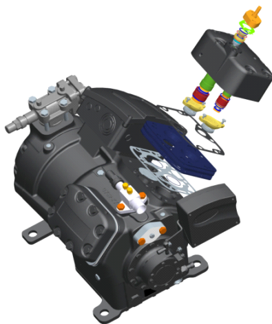
Figure 2: Exploded view of Digital mechanism
