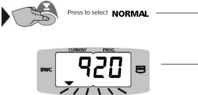
The left-hand section shows the current number of wraps and the right hand section shows the target number. When the current number = Target number, the alarm will sound for 2 seconds and the display will flash. (If set, the early warning alarm sounds beforehand). Automatic reset of current number to zero normally occurs 5 seconds after the Target number is reached. If additional wraps are added after the Target number is reached, the current number will continue to advance.
