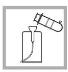
**19.** Pour the filtered, reacted sample from the plunger reservoir into the Pour-Thru Cell.
