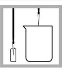
4. Use a TenSette<sup>®</sup> Pipet to add 1.0 mL of Blanking Reagent to the beaker. Swirl several times to mix.
