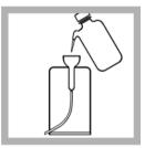
**20.** Flush the Pour-Thru Cell with at least 50-mL of deionized water immediately after use.
