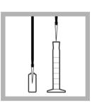
7. Use a TenSette Pipet and a clean tip to transfer 1.0 mL of buffer from the ampule a clean 50 mL mixing graduated cylinder.
