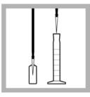
6. Using a TenSette<sup>®</sup> Pipet and a clean tip, transfer 1.0 mL of buffer from the ampule to a clean, treated 50-mL graduated mixing cylinder.
