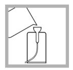
**12.** During the reaction period, flush the Pour-Thru Cell with the remainder of original dechlorinated water from step 10.
