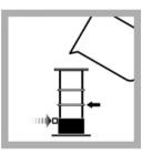
11. Push the valve button on the OriFlo<sup>™</sup> barrel assembly in ("closed" position). Place the barrel assembly into its stand. Pour approximately 50 mL of the original sample into the barrel.
