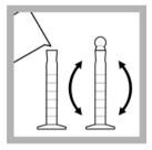
9. Prepared Sample: Avoiding extra agitation, carefully fill the cylinder to the 50-mL mark with sample. Stopper the cylinder. Gently invert it twice to mix.
