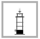
**12.** Insert the plunger into the barrel and slowly push the plunger down with even pressure, until the plunger is fully seated.
