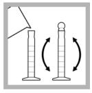
**10.** Fill the cylinder to the 50-mL mark with dechlorinated water from step 4. Cap and invert twice to mix. Save the remaining water for step 12.
