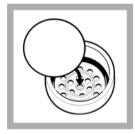
4. Install a new, 3-micron filter (white) into the cap well. Wet the filter with a few drops of deionized water. Reassemble and hand-tighten the cap onto the plunger.
