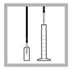
**9.** Use a TenSette Pipet and a clean tip to transfer 1.0 mL of indicator from the ampule to the cylinder. Swirl to mix the reagents. Proceed to step 10 within one minute.
