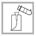
**13.** Pour the filtered sample from the plunger reservoir into the Pour-Thru Cell.
