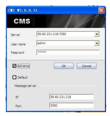
Sever IP is the IP of the PC installed transmit sever, if transmit sever is in LAN with CMS client, the sever IP should be LAN IP. If you connect to sever via WAN, then the IP should be public IP. If the message server and the transmit server are on the same PC, and the port is default 5556, then you can tip Default. Otherwise, please input the message server and port below.
