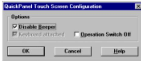
Note the addition of a new checkbox labeled *Operation Switch Off*. The Hand Held is equipped with an OP (operation) keypad on the front of the unit, and a finger switch (sometimes known as dead man switch) located on the back under the left hand grip. Pressing either switch will enable the touch screen. Checking the *Operation Switch Off* will disable the switch function and the touch screen will always be enabled.
