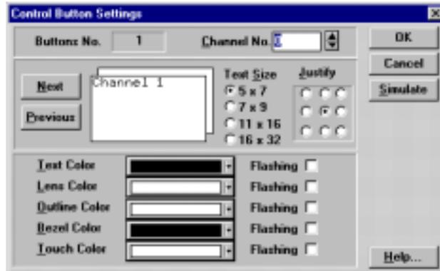
The *Buttons No.* information box displays the assigned button number. The *Channel No.* list box selects the video source for the assigned button. Each button can select from CH0, CH1, or CH2. Although the spin controls allow selection of CH3, it is not used in this product.
