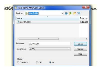
After the file being transferred. You will get a message like this "Firmware has been updated successfully. Version 1.0.2." After that you can release the boot loader mode and reset the chip, or run R command to run the firmware.
