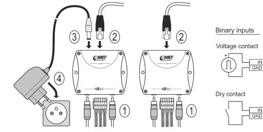
Binary inputs terminals connection procedure:
