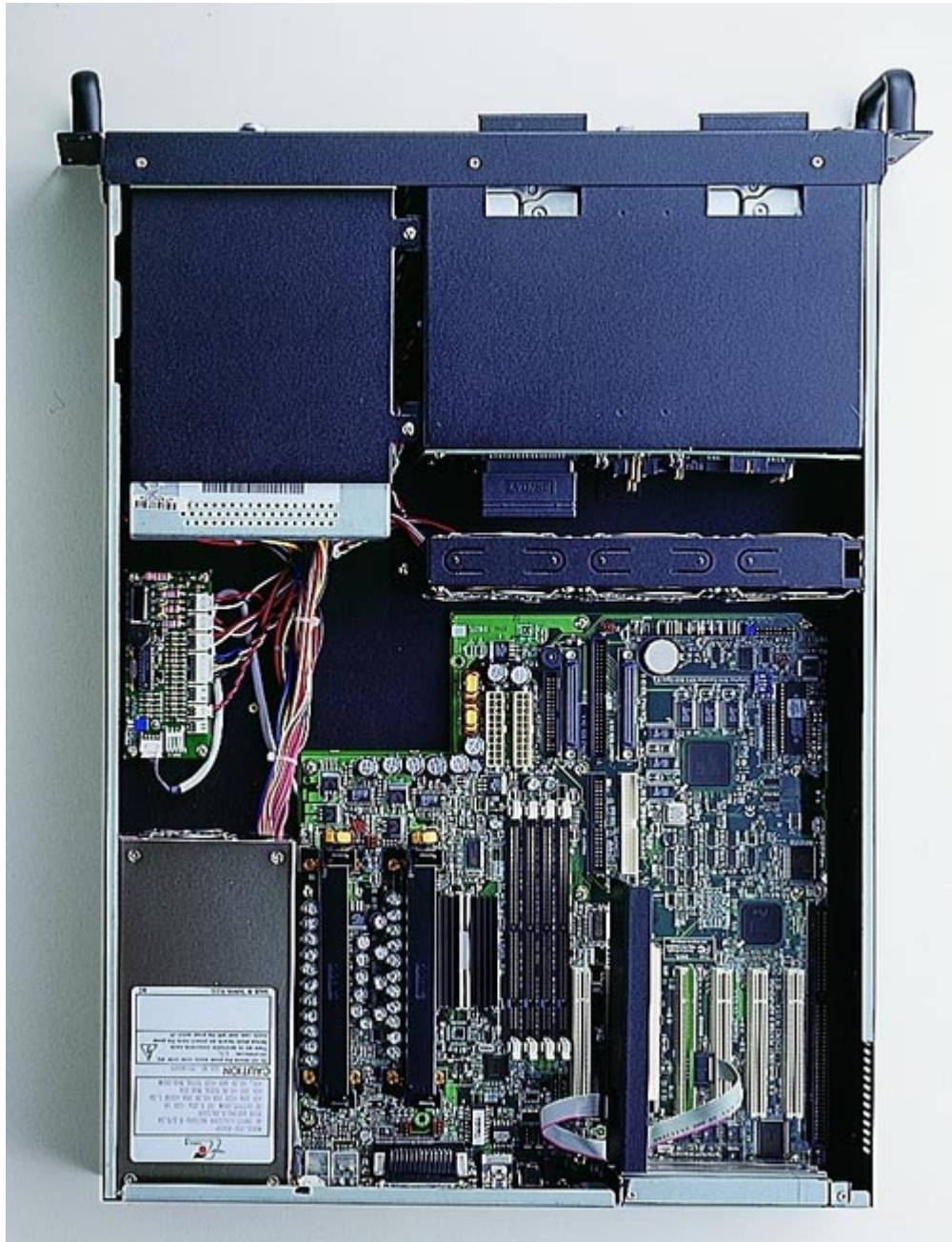
Figure 2-3: IPC-613 with server motherboard
