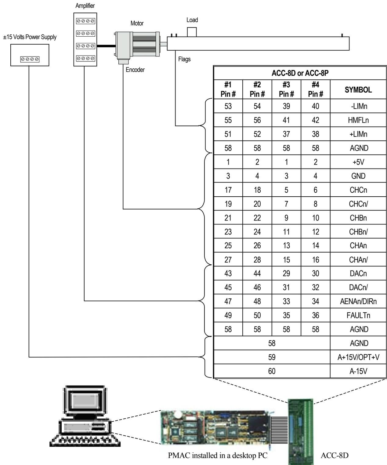
This diagram is just an example of one of the many variations of the machine connections. PMAC Jumpers must be set appropriately following both the appropriate PMAC Hardware Reference and the PMAC User's Manual.
