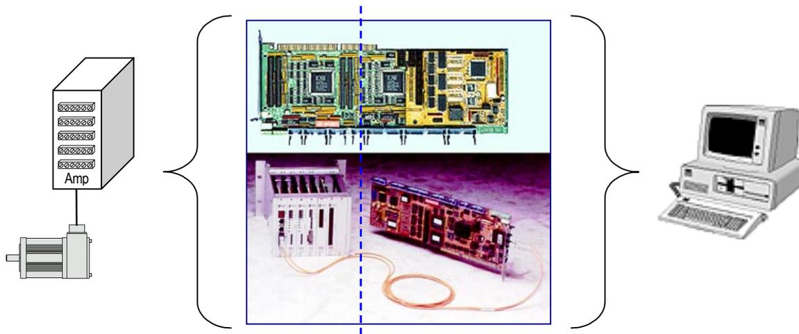
The PMAC2 and the MACRO (Motion And Control Ring Optical) stations are linked with a fiber optic or twisted pair connection. This clever distribution of components brings many benefits: drastic reduction of wiring complexity, elimination of interference by electromagnetic noise and long distance connections (3000 m, ~2 miles with glass fiber).
