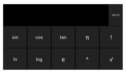
In the basic panel, you can enter the "advanced panel" either by selecting the "advanced panel" after touching the "Option " button, or sliding your single finger from right to left; In the advanced panel, you can return to the "basic panel" either by selecting the "basic panel" after touching the "Option" button, or sliding your single finger from left to right.
