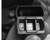
When the battery has been installed, check that the battery housing and O-ring are clean. The O-ring must always be lubricated with a thin layer of silicone lubricant.
