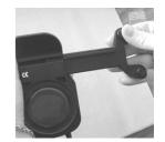
Attach the NACS<sup>TM</sup> to the mask by positioning the holes of the transparent part over the black buttons of the clamping band and pressing. These buttons are the same ones that hold the protective shield when the mask is not in use. Make sure the protective shield is removed prior to attaching the NACS<sup>TM</sup> to the mask.
