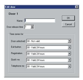
4. Find a name for the door and type it in the **Name** field. Note that this name will not be stored in the central unit, so if another PC connects to the central unit, this name will not be shown on that PC.
