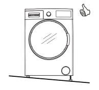
You can adjust the balance of your machine using a level from the top.
