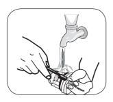
• Clean the foreign materials inside the filter with the help of a brush.
