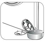
• Pull the black rubber hose and detach it from its clamp, place a container under it and remove its plug.
