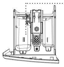
Main wash detergent compartment: In this compartment, only materials like detergent (liquid or powder) or anti-lime. You can find the liquid detergent apparatus for your liquid detergent inside your machine during
