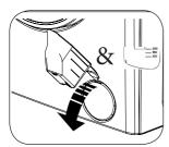
• You may use the washing powder scoop supplied with your machine or liquid detergent level plate to open the pump cover.
