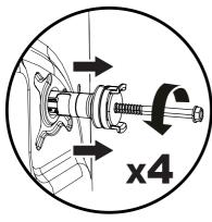
Transport screws should then be removed by pulling them out. The removed transport safety screws should be stored to be used again in case the machine needs to be transported in the future, e.g. if moving house.
