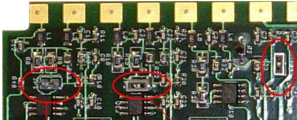
Input 1 with no jumper - set for Temperature
