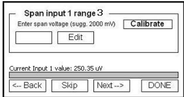
The current value is displayed directly above the bottom row of buttons as Current Input 1 value: XX.X uV.
