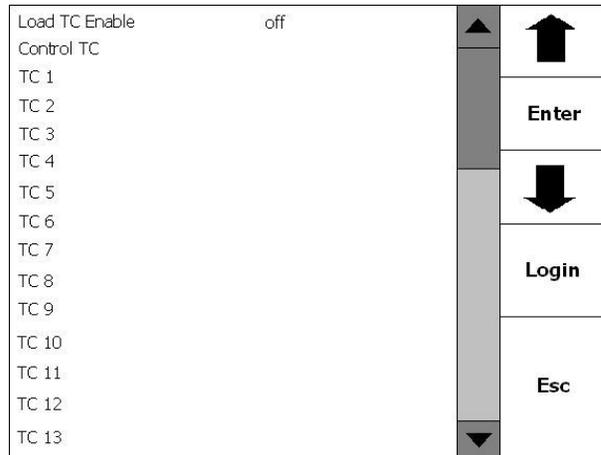
To activate one or more of the thermocouples, use the blue up and down arrows to highlight the desired thermocouple then press **Enter**. This will activate, or deactivate the selected thermocouple.
