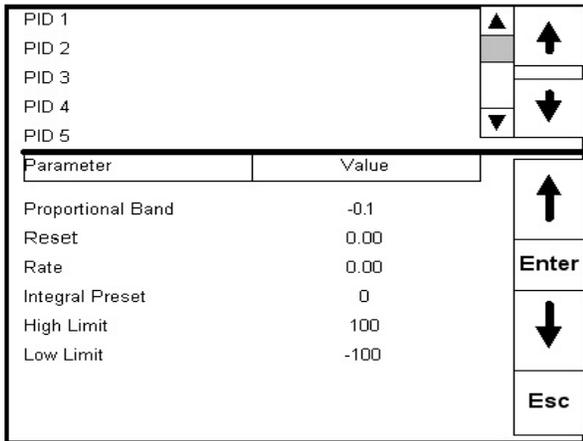
This screen is used to enable up to 16 sets of alternate PID's for control purposes. It is implemented with the PID Select Opcode in the program.
