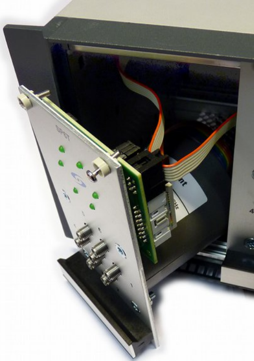
Figure 11: Flat ribbon cable on a SP6T module
