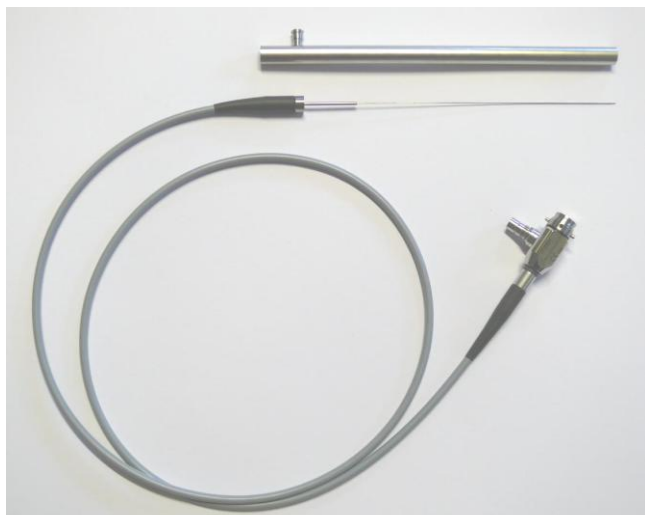
Figure 1 – Dental Modular Endoscope with protective tube for optic
