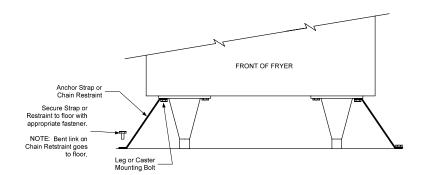
**NOTE**: If you need to relocate a fryer installed with legs, remove all weight from each leg before moving. If a leg becomes damaged, contact your service agent for immediate repair or replacement.
