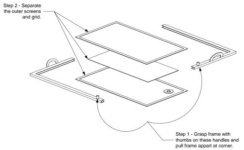
2. Separate the outer screens and grid.
