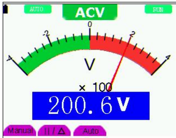
figure 26: AC Voltage Measurement
