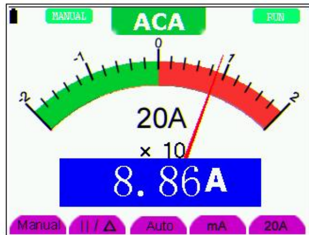
figure 30: AC Current Measurement for 20A
