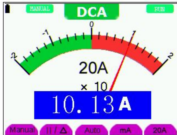
figure 28: DC Current Measurement for 20A
