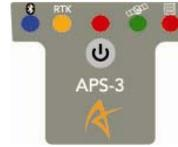
Press ON/OFF button to turn ON APS-3. Hold ON/OFF switch for 5 seconds to turn OFF APS-3.
