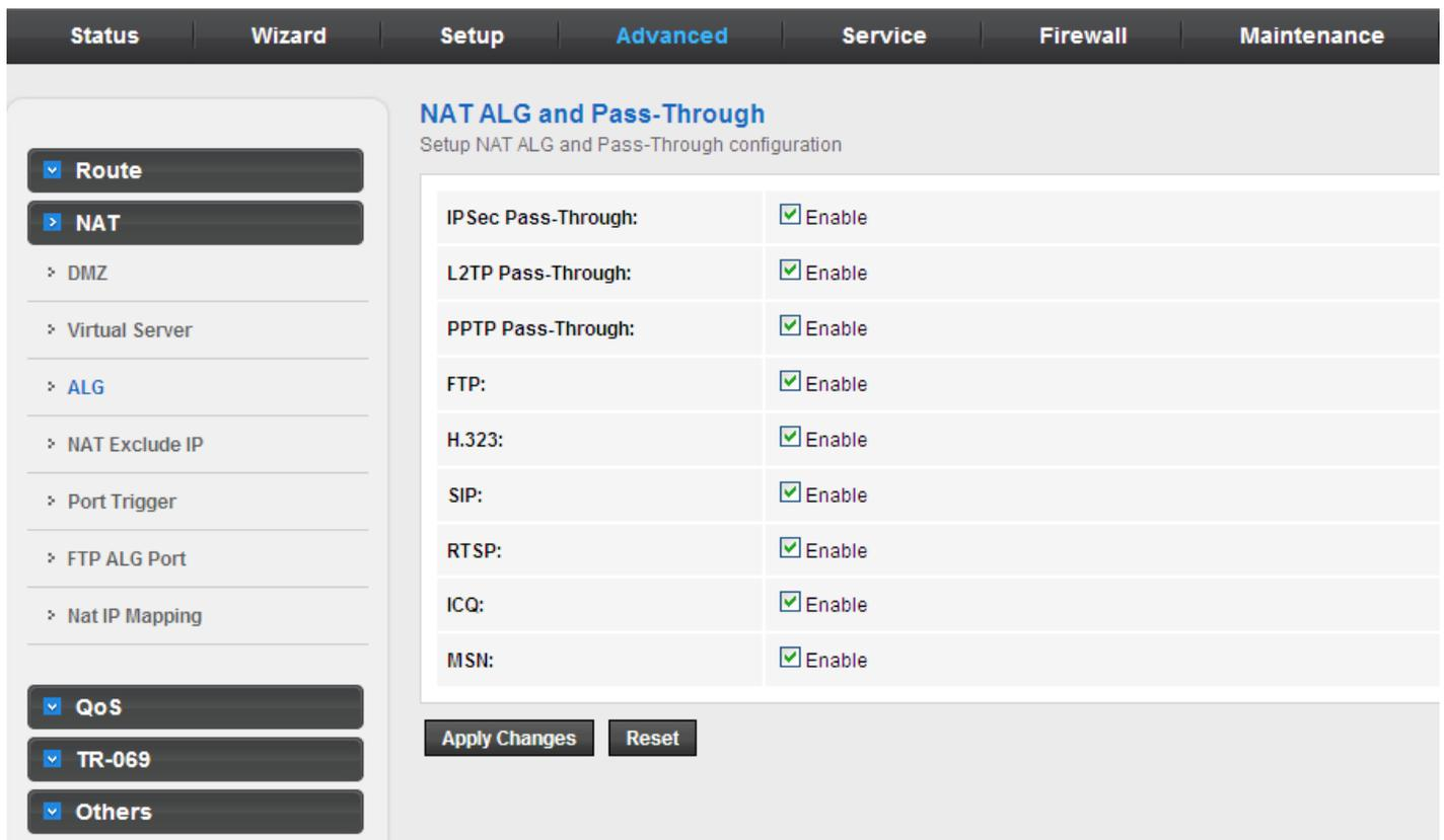
The screenshot shows the 'NAT ALG and Pass-Through' configuration page. The navigation menu on the left includes 'Route', 'NAT', 'DMZ', 'Virtual Server', 'ALG' (selected), 'NAT Exclude IP', 'Port Trigger', 'FTP ALG Port', and 'Nat IP Mapping'. Below the menu are sections for 'QoS', 'TR-069', and 'Others'. The main configuration area is titled 'NAT ALG and Pass-Through' and contains the following settings:
