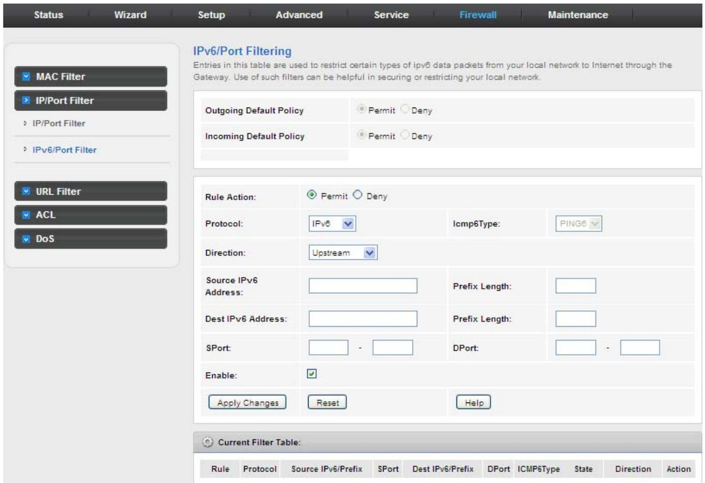
The screenshot shows the 'IPv6/Port Filtering' configuration page. The left sidebar contains navigation options: MAC Filter, IP/Port Filter (selected), URL Filter, ACL, and DoS. The main content area is titled 'IPv6/Port Filtering' and includes a description: 'Entries in this table are used to restrict certain types of ipv6 data packets from your local network to Internet through the Gateway. Use of such filters can be helpful in securing or restricting your local network.'
