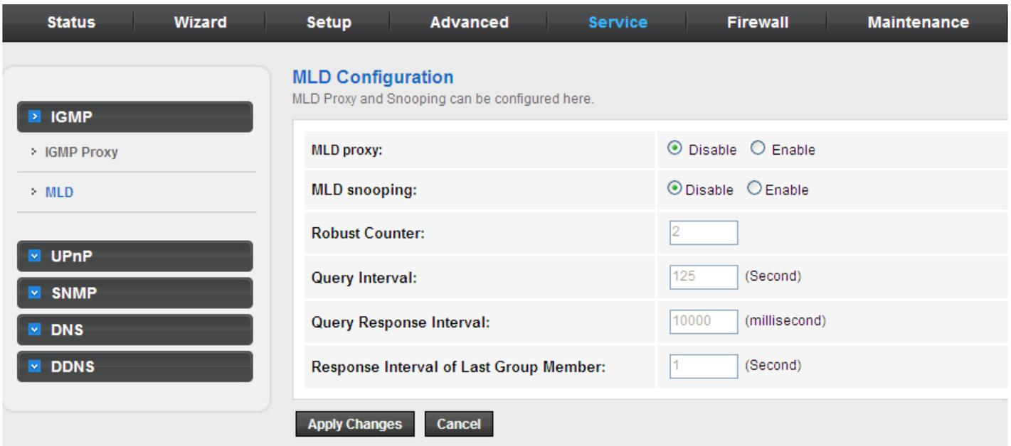
The screenshot shows the 'Service' tab in the router's configuration interface. The left sidebar contains a tree view with 'IGMP' expanded to show 'IGMP Proxy' and 'MLD'. Below this are buttons for 'UPnP', 'SNMP', 'DNS', and 'DDNS'. The main content area is titled 'MLD Configuration' and includes the instruction 'MLD Proxy and Snooping can be configured here.' The configuration table is as follows:
