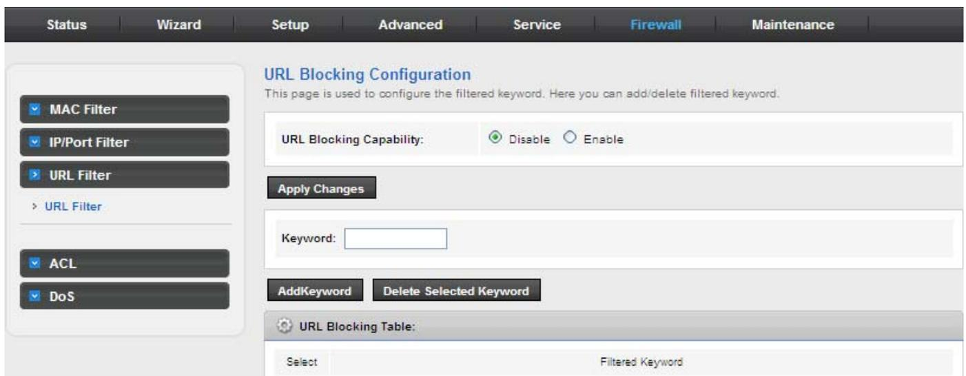
The screenshot shows the 'URL Blocking Configuration' page. The left sidebar contains navigation options: MAC Filter, IP/Port Filter, URL Filter (selected), ACL, and DoS. The main content area is titled 'URL Blocking Configuration' and includes a description: 'This page is used to configure the filtered keyword. Here you can add/delete filtered keyword.'
