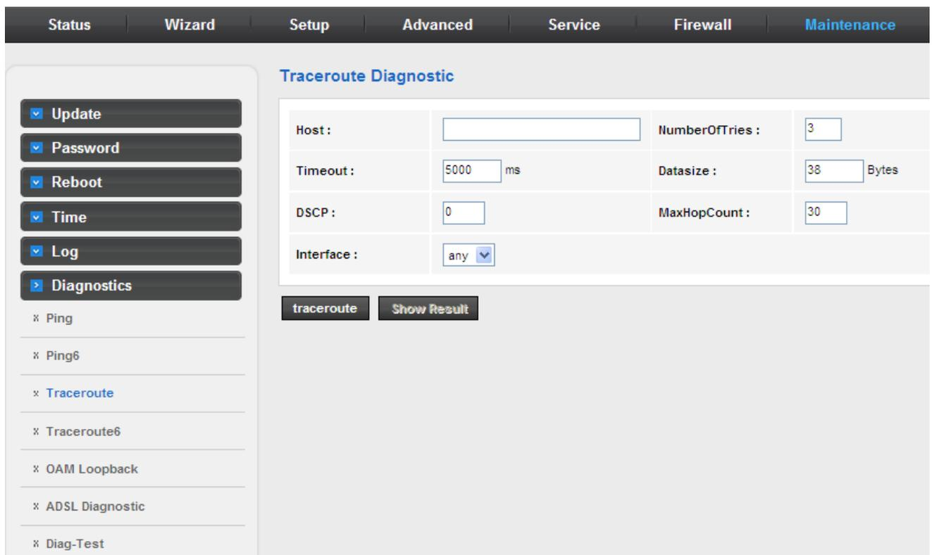
The screenshot shows the router's web interface with the 'Maintenance' tab selected. On the left, a sidebar menu under 'Diagnostics' has 'Traceroute' highlighted. The main content area is titled 'Traceroute Diagnostic' and contains the following fields:
