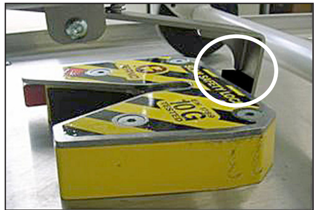
Figure 22 - Stop Bar Lowered
