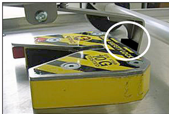
Figure 8 - Stop Bar Lowered During Improper Unloading
