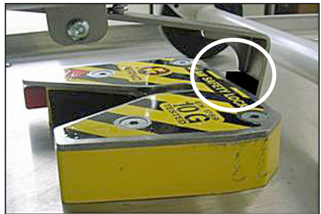
Figure 3 - Stop Bar Catching Fastener
