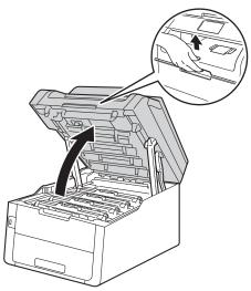
2 Remove the toner cartridge and drum unit assembly.
