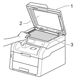
4 In the ADF unit, clean the white bar (1) and the scanner glass strip (2) underneath it with a soft lint-free cloth moistened with water.
