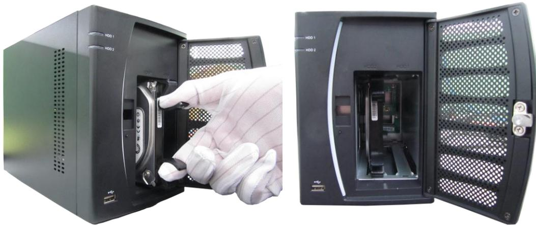
5. Repeat the above steps to install other hard disks onto the NVR. After having finished the installation of all hard disks, close the front panel and lock it with the key again.
