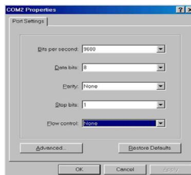
Figure 4-5. Communication Parameters
