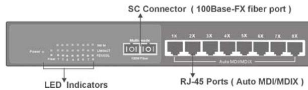
Figure 3-3. Front Panel of the 1008-MSC Switch
