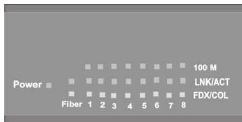
Figure 3-5. LED Indicators for 1008 Switch
