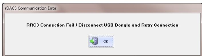
Should you fail to establish a Host Mode session, switch off all power sources, double check all your connections, physically disconnect and reconnect the USB IO dongle, then restart the connection sequence again as described above.
