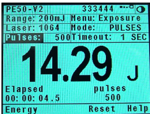
Figure 6.2. Exposure Screen set to stop after summing 500 pulses
