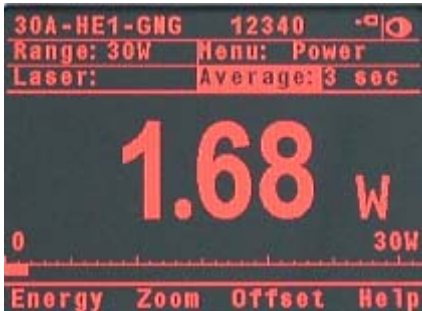
Figure 4.2. Thermopile Power Screen with average set to 3 seconds
