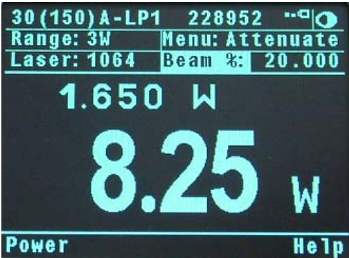
Figure 4.8 Attenuation Screen with Beam % set to 20%
