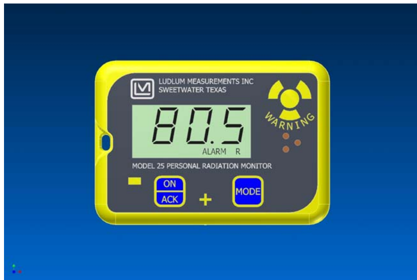
Figure 2: Accumulated Dose Screen with ALARM indicator
