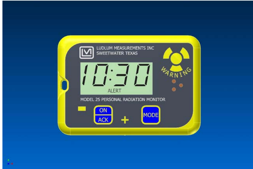
Figure 3: Time Remaining Screen with ALERT indication
